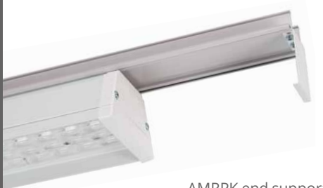
AMRPK end support and lower bracket which can be fastened by screw or by pressing together must be ordered separately. With the lower bracket the ramp luminaires installed between the lighting suspension rails can be positioned on the same level as luminaires installed to the lighting suspension rail with AMJK2 spring brackets.
