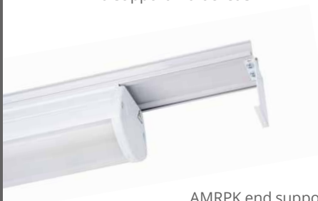
AMRPK end support and lower bracket which can be fastened by screw or by pressing together must be ordered separately. With the lower bracket the ramp luminaires installed between the lighting suspension rails can be positioned on the same level as luminaires installed to the lighting suspension rail with AMJK2 spring brackets.
